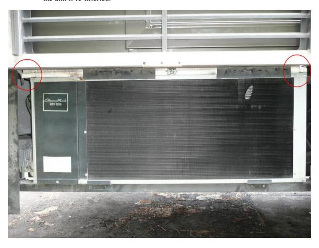
25. Re-install the duct, first attaching the two bottom screws, one on each side from under the coach, but don't tighten. Then as the picture shows, use a short screw driver to put in the two top screws and on the outside, it can be done looking thru from the side. After all ten screws are started, and then tighten all.
