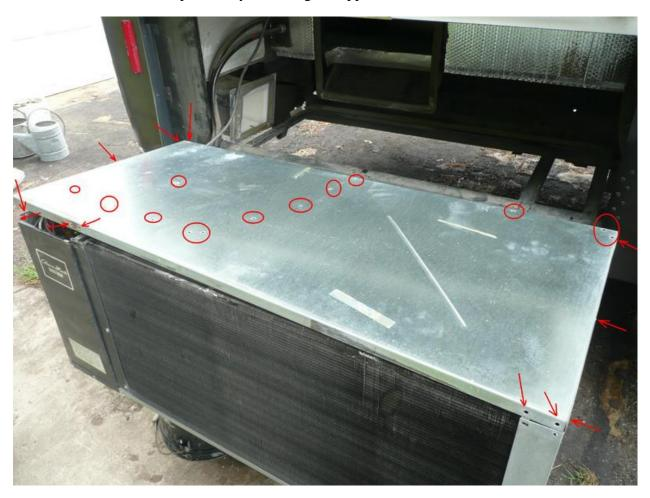
13. Remove these two additional screws to allow the condenser coil to be opened at the top if you need to pull the outdoor blower assy.
