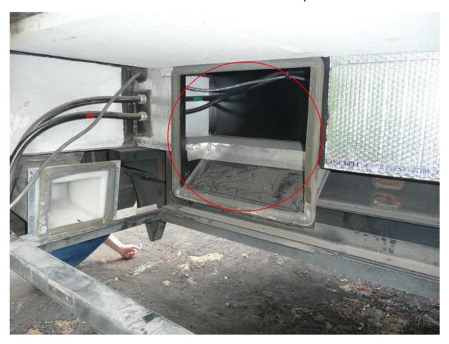
23. Reinstall the top cover using the approx 28 screws. Use a pointy object like an awl to align some of the holes in the middle of the top panel. Put the two screws back in front of the right side panel. Slide the entire unit back in coach. Once the unit is partially in, then feed the power cables up and over the duct. Re-install the four brackets.
