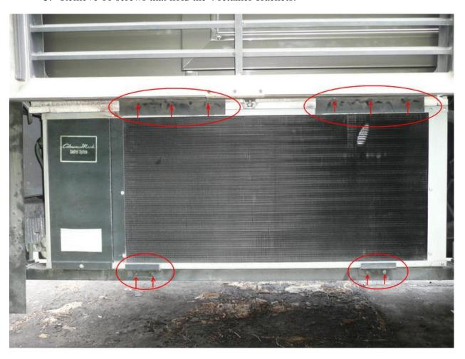
4. Remove 5 screws on left side of the cold air output duct. Good news is that there are no screws across the top!
