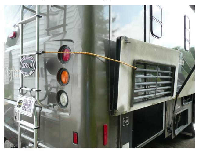
3. Remove 10 screws that hold the 4 retainer brackets.
