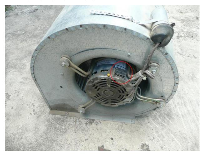
18. To replace the motor and/or squirrel cage, remove the 4 ea screw & nuts. Disconnect the two brown wires from the starting cap. Note the brown/white connects to the bottom spade lug (behind the rubber cover). Also note the motor bracket is not symmetrical & when re-assembling, make sure the wire connector is at the top.
