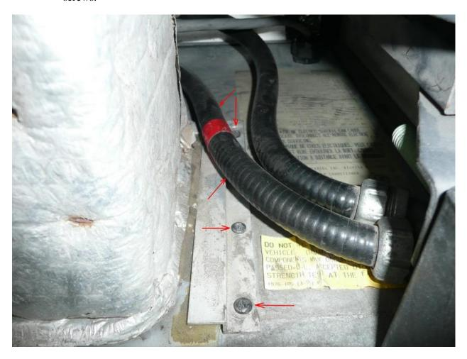
6. Remove (or loosen) the 2 screws if it is possible (if not too corroded). These sheet metal screws are going into heavy angle iron and can be difficult to remove. It may be possible to remove A/C unit without messing with this bracket. I was able to back out 3/8 inch & that allowed plenty of clearance.
