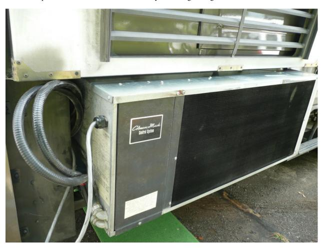
10. Support the unit off the ground to make it easy to carry, work on, and test while still keeping all the cables connected. I built a bench from two 5 gal buckets and two 2x6 planks. This was plenty strong and stable. Earlier in the campground I used the bench part of a picnic table. Leave open space under the Outdoor Blower screen so you can run the unit with the top panel off and test everything before closing up.
