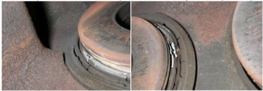
Heat damaged ABS system wheel speed sensors
