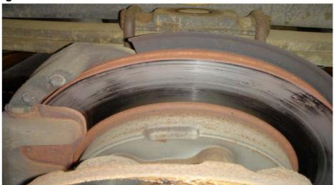
The rotor shown below exhibits severe brake pad material transfer and is a good indicator that the brake caliper assembly at this wheel end had experienced brake drag that may be related to the safety defect. The excessive amount of brake pad material transferred on to the rotor would be considered collateral damage and will require the replacement of the rotor. The associated cost is covered by the interim repair procedure if a caliper failure has occurred.
