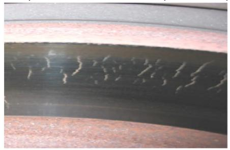
The existence of cracked rotors as described above, and without any other evidence (see additional items described below), would not justify a caliper replacement per the interim letter – neither would the replacement of the rotor qualify for a goodwill policy replacement. A replacement of the rotor under these conditions would be the responsibility of the customer.
