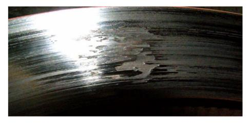
Note: If the only evidence or complaint by the owner is a cracked rotor or one that exhibits slight to moderate brake pad material transfer – this is NOT sufficient evidence of a related brake caliper piston sticking condition.
