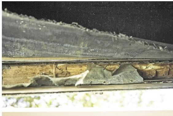
I believe we can successfully treat the rot and then re-build about 60% of the wood with epoxy putty. I will attempt to replace the balance of the wood with new treated lumber and some more of the epoxy putty. When that is done, I will fiberglass the rear side up to the floor and then finish the bottom off with the original plastic channel trip.
