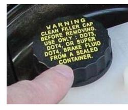
When the fluid is changed, use the type of brake fluid (**DOT 3 or 4**) specified by the vehicle manufacturer. The cap on the fluid reservoir will usually indicate what type of brake fluid is required. You can also find this information in your **Owner's** Manual (look under brake fluid).
