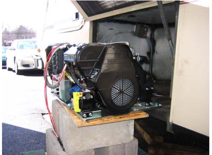
This is a view of the empty generator compartment. The openings in the floor are for cooling needs, service drain access, etc. Sound deadening material lines the compartment.
